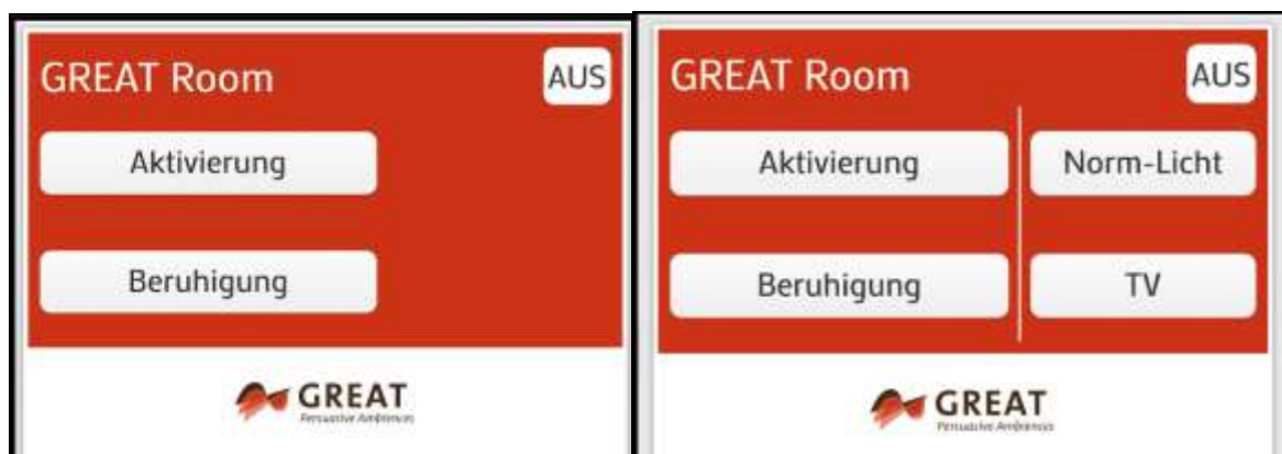
Figure 7: Different control options for the GREAT luminaire: basic functions (left), advanced functions (right)
