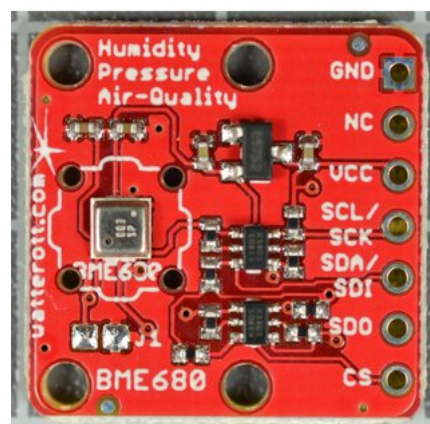
Figure 66: Watterott Bosch BME 680 breakout board
